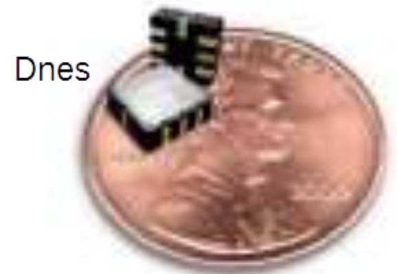
The first commercial accelerometer from Analog Devices (1990); 10 x 10 mm
