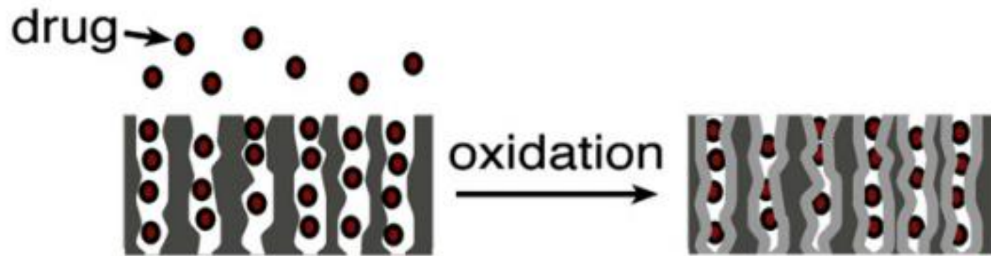
Fig. 4. Building a bottle around a ship. A molecular or nanoparticle payload can be trapped by partial oxidation of the porous Si host layer. Oxidation produces a volume expansion (Si to SiO 2 ) that shrinks the pores, locking the payload in place. After [124].
