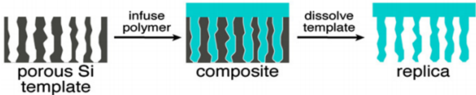
Fig. 6. Fabrication of a nanostructured composite from a porous Si template. A variety of solution- or melt-processible organic and biopolymers can be solution-cast or injection-molded into a porous Si or porous SiO 2 host. The composite can be used as-formed, or the template can be removed by chemical dissolution. If the template is removed, the polymer castings often replicate the nanostructure of the master. Use of these castings as vapor sensors, deformable and tunable optical filters, and as self-reporting, bioresorbable materials has been demonstrated [146].
